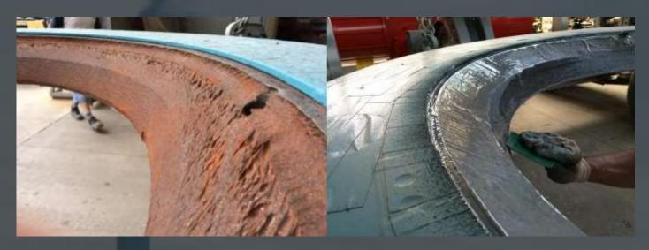
DENSIQ manufactures a range of solvent free epoxy repair products that contain hardened ceramic beads.
